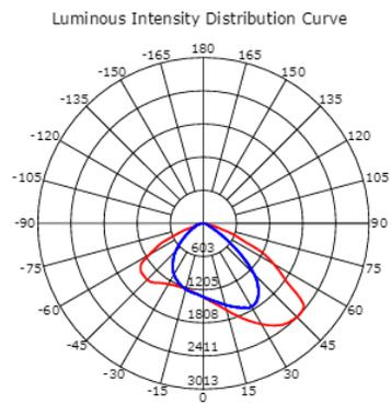
Beam Angle(50%) C0-180,C90-270: 122.6 deg,89.2 deg
